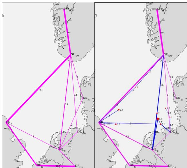
Figure 3. Accumulated transmission investments and hub investments by 2050. Radial Case (left) vs Meshed Case (right)
