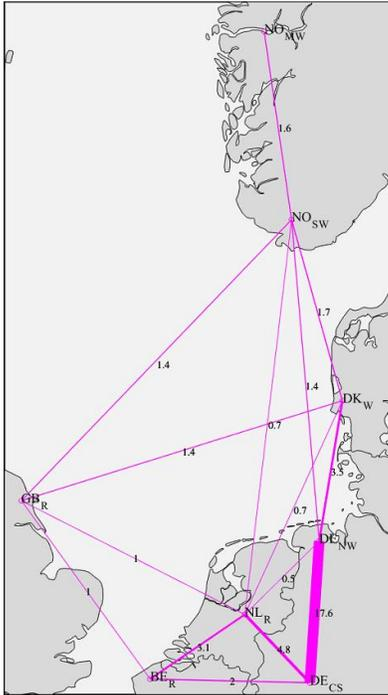
Figure 1. Exogenous transmission capacities (GW between regions most relevant to the North Sea area (connection points to the onshore power systems are not the actual locations)). DK\_W to DE\_NW is an onshore line
